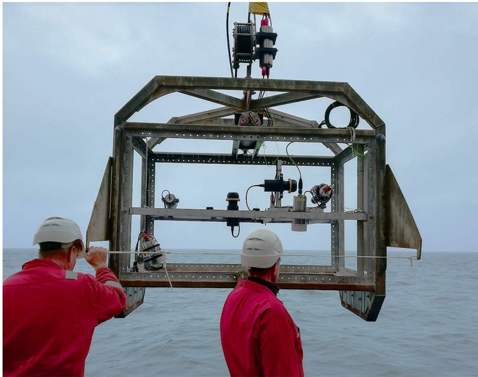
Figure 4. Front view of the NIOZ hopper camera.
