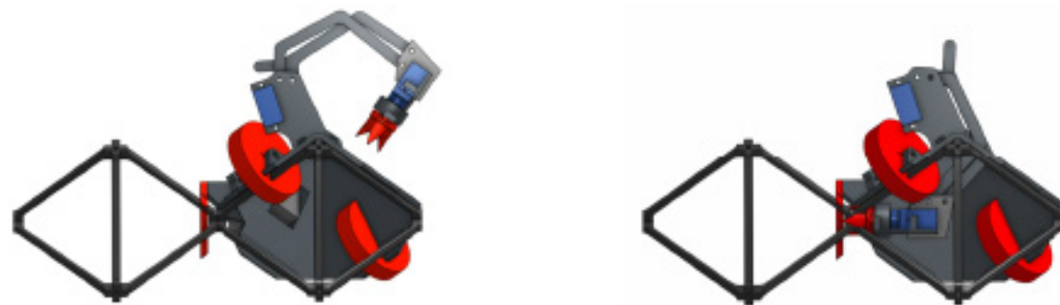
Figure 10. Robot end effector by Luijten. (L) Initial position (R) Connection position (Luijten, A., 2020)
