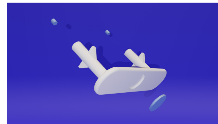
Figure 58. Overview of the magnets inside the pin bridge
