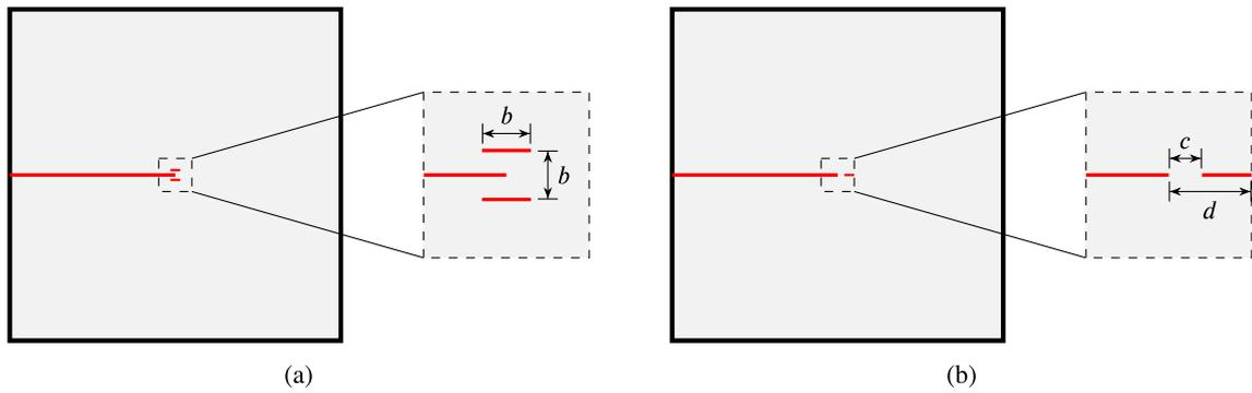
Fig. 14. (a) Shielding configuration; and (b) Amplification configuration.
