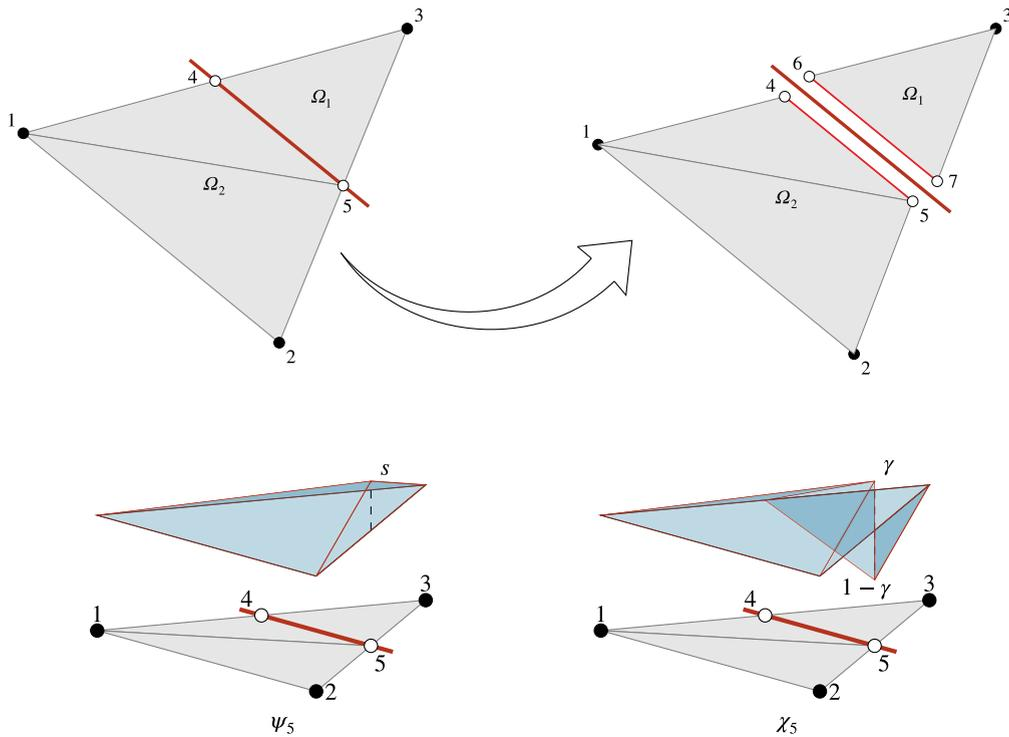
Fig. 2. (top) A triangular element with nodes 1, 2, 3 cut by a single discontinuity in standard FEM. The element is divided into two subdomains  $\Omega_1$ ,  $\Omega_2$ ; (bottom) Enrichment functions for a node along the discontinuity that reproduce the same kinematics. While the weak enrichment function  $\psi_5$  is continuous the strong enrichment  $\chi_5$  is discontinuous.
