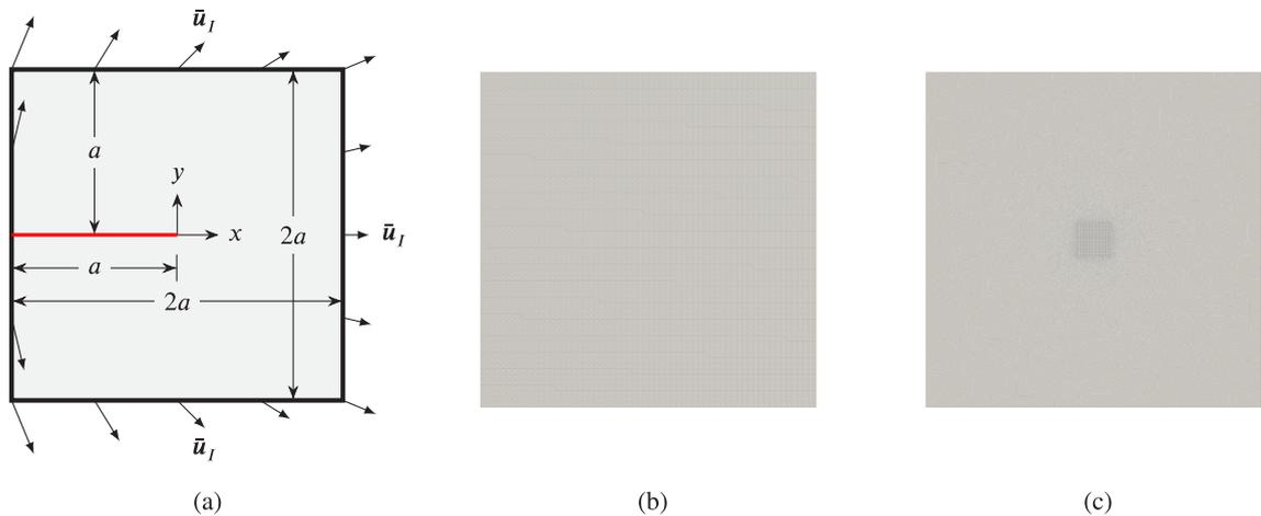
Fig. 13. An edge-notched plate subjected to mode I loading, thereby we prescribe an asymptotic displacement field  $\bar{u}_I$ ; (b, c) Finite element meshes used for the verification of crack shielding and amplification effects: (b) structured; and (c) unstructured refined mesh.
