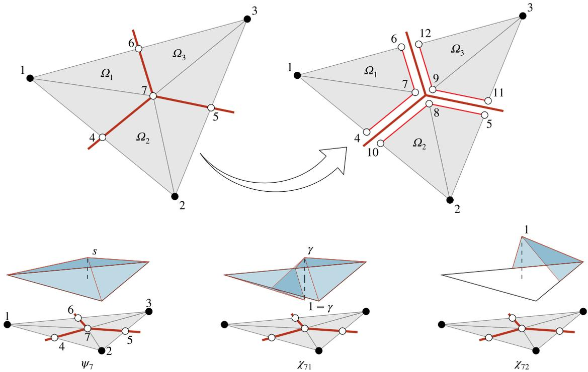
Fig. 4. (top) A triangular element with nodes 1, 2, 3 cut by three discontinuities in standard FEM norm. The element is divided into 3 domains  $\Omega_1, \Omega_2, \Omega_3$ . (bottom) Enrichment functions for a 3-fold junction node.  $\psi_7$ : The weak enrichment function,  $\chi_{71}$ : The first strong enrichment function,  $\chi_{72}$ : The second strong enrichment function.
