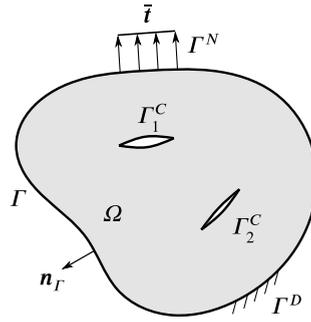
Fig. 1. A continuous body  $\Omega$  with boundary  $\Gamma$  having unit normal  $\mathbf{n}_\Gamma$ . The body contains multiple traction-free cracks  $\bigcup_{i=1}^n \Gamma_i^C \subset \Gamma$ . Boundary conditions include prescribed tractions  $\bar{\mathbf{i}}$  on  $\Gamma^N$  and prescribed displacements  $\bar{\mathbf{u}}$  on  $\Gamma^D$ .
