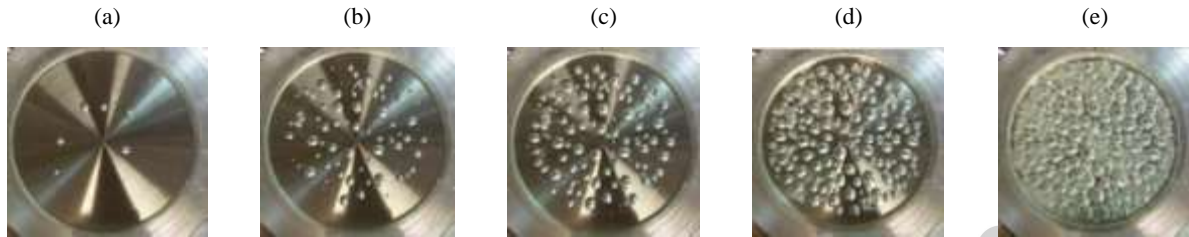
Figure 15: Evolution of cohesive bubble in SG laminated connection under tensile force (a) bubble formation (b-c) bubbles expand and new bubble are formed (d) distance between bubble is constant and number of bubble is stable (e) bubbles collapse and the remaining adhesive material form filaments that elongate
