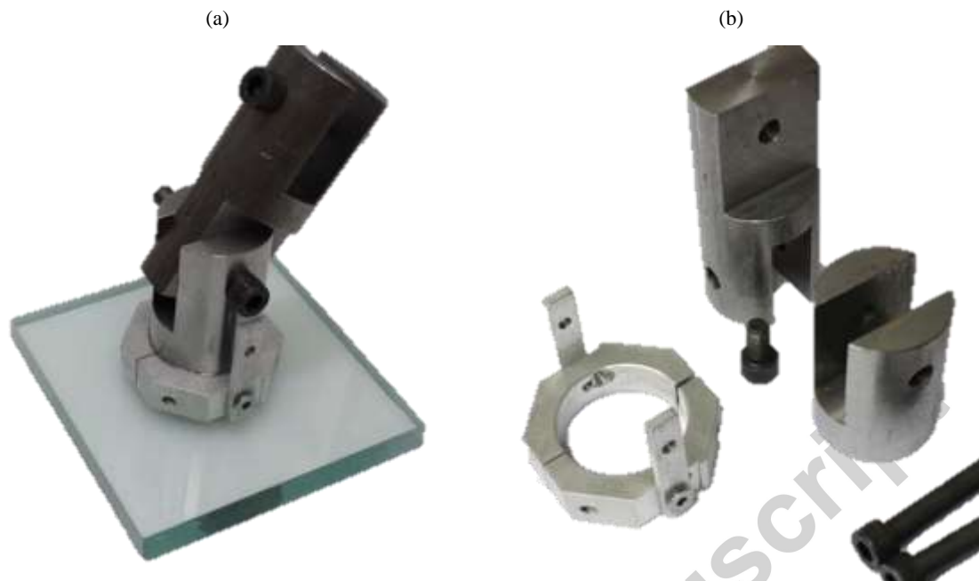
Figure 5: Photos of (a) a laminated connection with the metal fixture for LVDTs (b) exploded view
