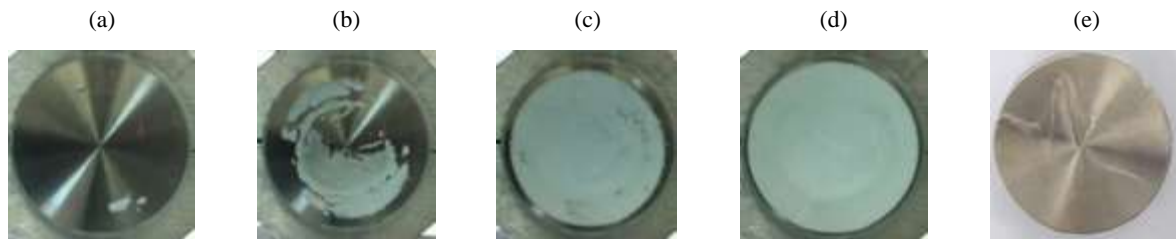
Figure 13: Evolution of whitening in TSSA laminated connection under tensile force (a) beginning (b) quick propagation over most of the adhesive (c) slow propagation close to the perimeter (d) full propagation with a transparent ring close to the perimeter (e) failure
