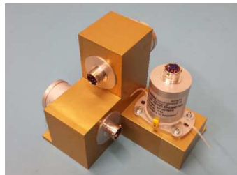
Figure 5.3: The angular accelerometers arrangement in an AAMU.
