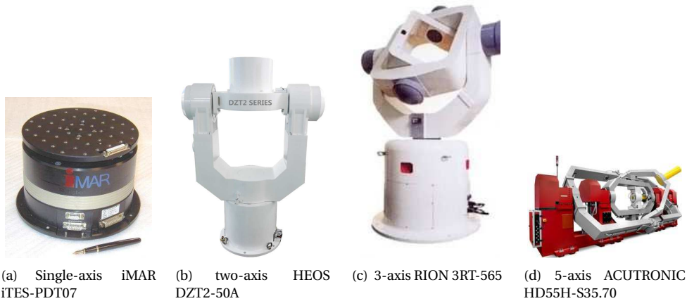
Figure 1.6: Motion simulator systems from iMAR GmbH 9 (a), Wuhan Huazhiyang Technology Co., Ltd 10 (b), Shenzhen RION Technology 11 (c), and ACUTRONIC 12 (d).
