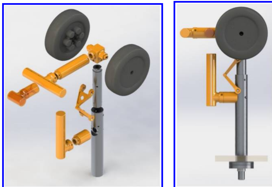
(a) LAGOON-SLG. D=150mm. Exploded view.
