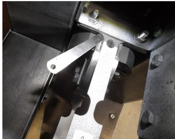
Figure 7.4: Clearance between drop tower and drop weight
