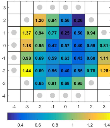
**Figure 4: Graphene sheet resistance.** Wafermap of the graphene sheet resistance [ $k\Omega$ ], with mean value of  $0.8 \pm 0.3 k\Omega$ . The grey circles mark broken devices. Part of the non-uniformity originates from the single zone heater of the CVD.
