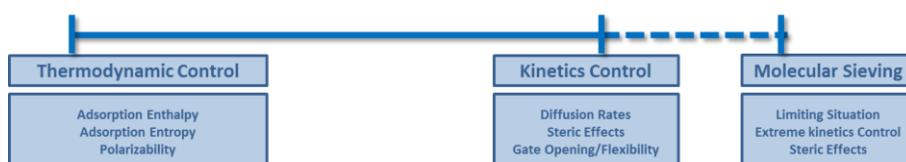
**Figure 5.** Adsorptive separation mechanisms scheme.
