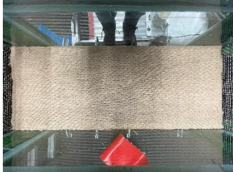
(c) Placement of geotextile
