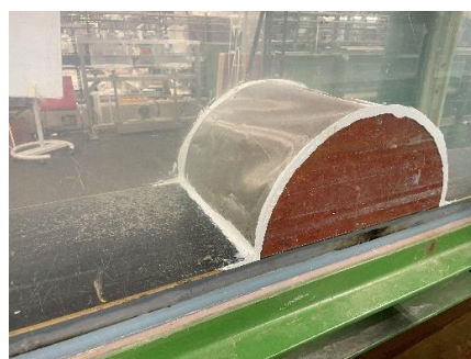
Figure 3-13: Sieve in the flume
