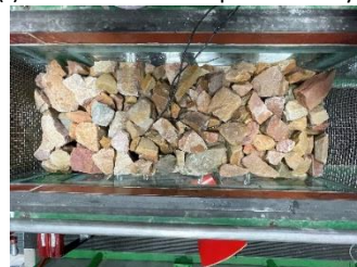
(h) Finishing filter layer
