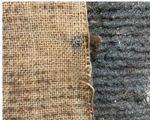
Figure 3-4: Support of jute on sandbed (left) and mechanically bonded fibers on filter layer side (right)
