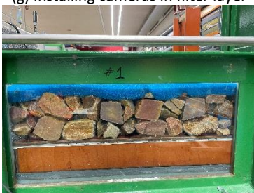
(i) Placement of rubber foam
