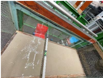
(a) Smoothen sandbed and if necessary, adding sand
