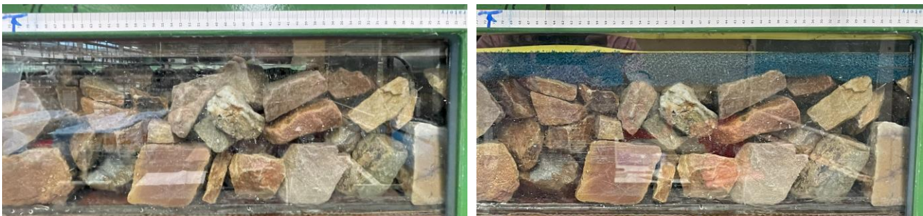
Figure 3-12: Filter layer without rubber foam (left) and filter layer with rubber foam (right)
