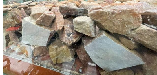
Figure 3-8: Cut stone placed against the side
