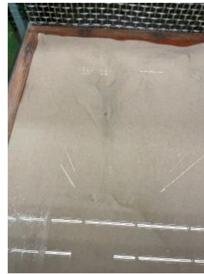
Figure F-34: Erosion channel
