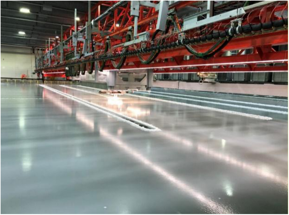
Fig. 3. Overview image taken during the experiments, showing the bridge spanning the ice tank and the carriage mounted under the bridge.
