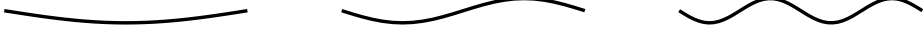
Figure 2.15: Three sine waves with the same amplitude, from left to right: \zeta(x) = -\zeta_0 \sin(ax) , a = 1, 2, 4 , x \in [0, 1] , \zeta_0 = 1/20 .
