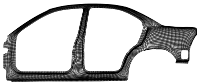
(a) Mesh of the geometry stored in car.off . The mesh consists of 31086 edges, 15895 vertices, and 62172 faces.
