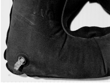
(c) Wrinkling in inflatable neck pillow, a classical example of wrinkling in a pressurised membrane.
