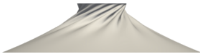
(a) Side view of the deformed annulus using the Kirchhoff-Love shell model.
