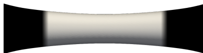
(b) Side view of the deformed annulus using the tension field theory membrane model. The black region denotes a taut region, and the grey region denotes a wrinkled region.
