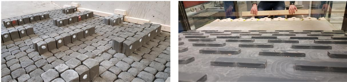
Figure 4.3: Different shape of ribs in Delta flume (left) and Scheldt flume (right)
