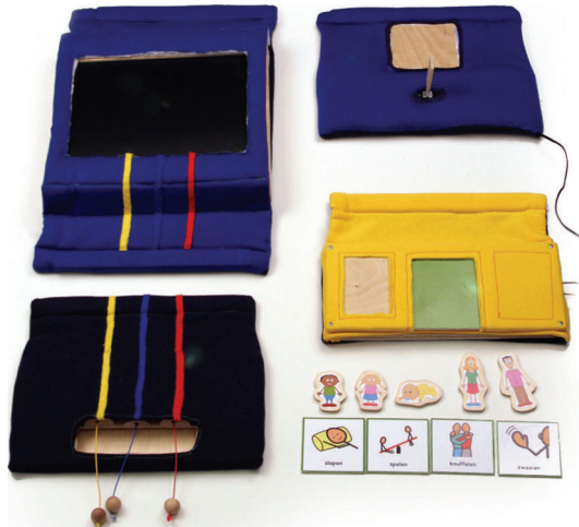
FIGURE 3: The KLEEd prototype, with clockwise from the top left: the console, the navigation mat, the combination mat, tagged input material, and the hide and seek mat.
