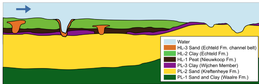
Fig. 1. Conceptual longitudinal subsurface lithological longitudinal section of a river bed, with typical distances of 10 to 20 m in depth and 10 to 20 km in length. Arrow indicates flow direction. In colour the lithological formations (Fm.) and members are indicated. Scour holes form in layers or patches composed of sandy material with lower erodibility compared to the surrounding resistant clay or peat layers.
