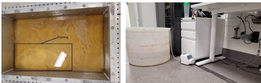
Figure 3.9: Saturating using centrifuge (a) Piping failure (b) Connection provided to pump fluid
