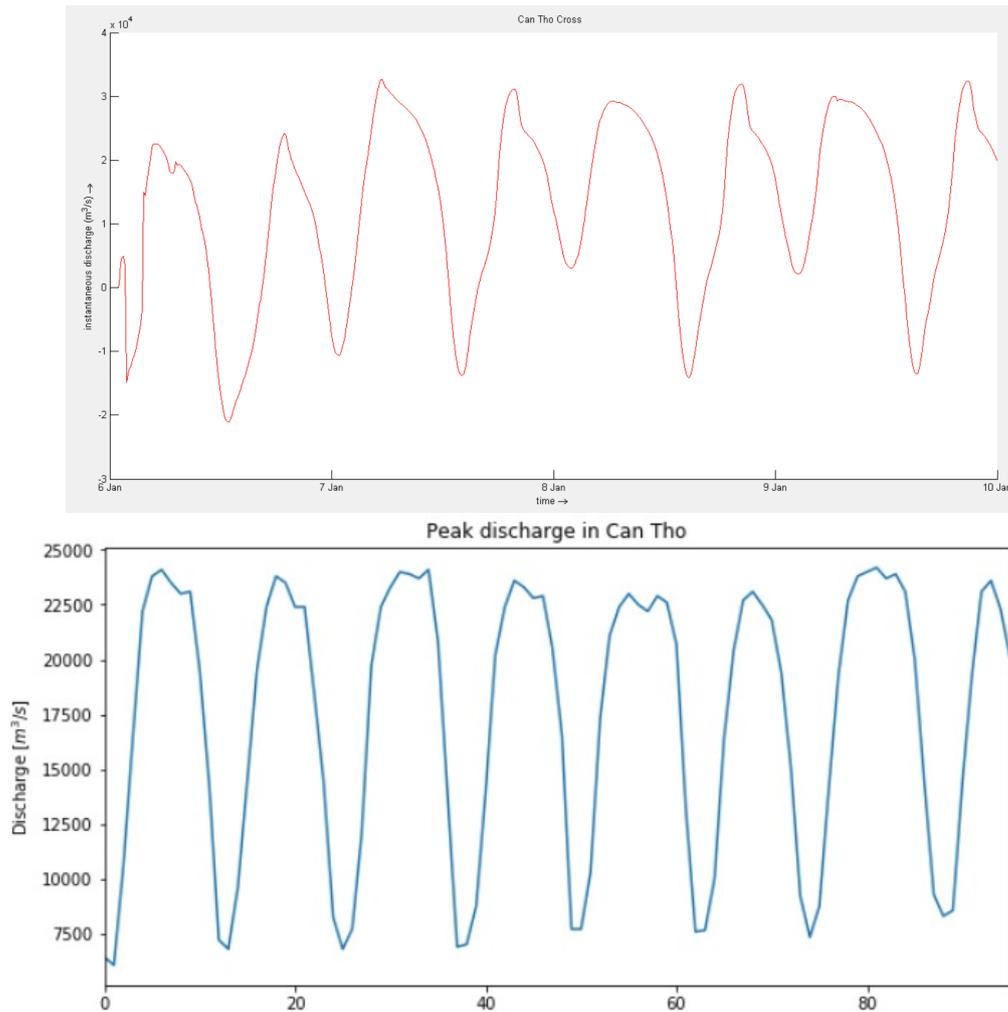
Figure 4.11: Validation discharge output Delft3D with measured data
