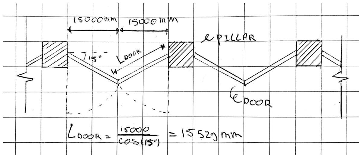
Figure I.1: Schematisation of the discharge sluice top view
