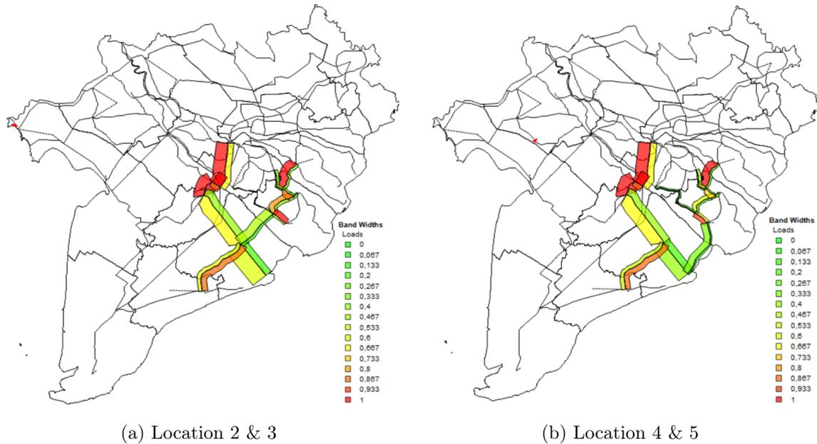
Figure 6.6: Network load for discharge sluice solution
