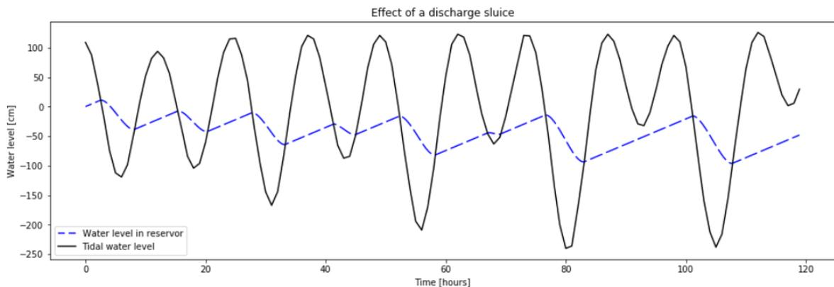
Figure 4.7: General scheme of the effect of a discharge sluice
