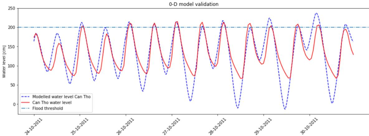
Figure 4.5: Calculated water levels in Can Tho for a part of October
