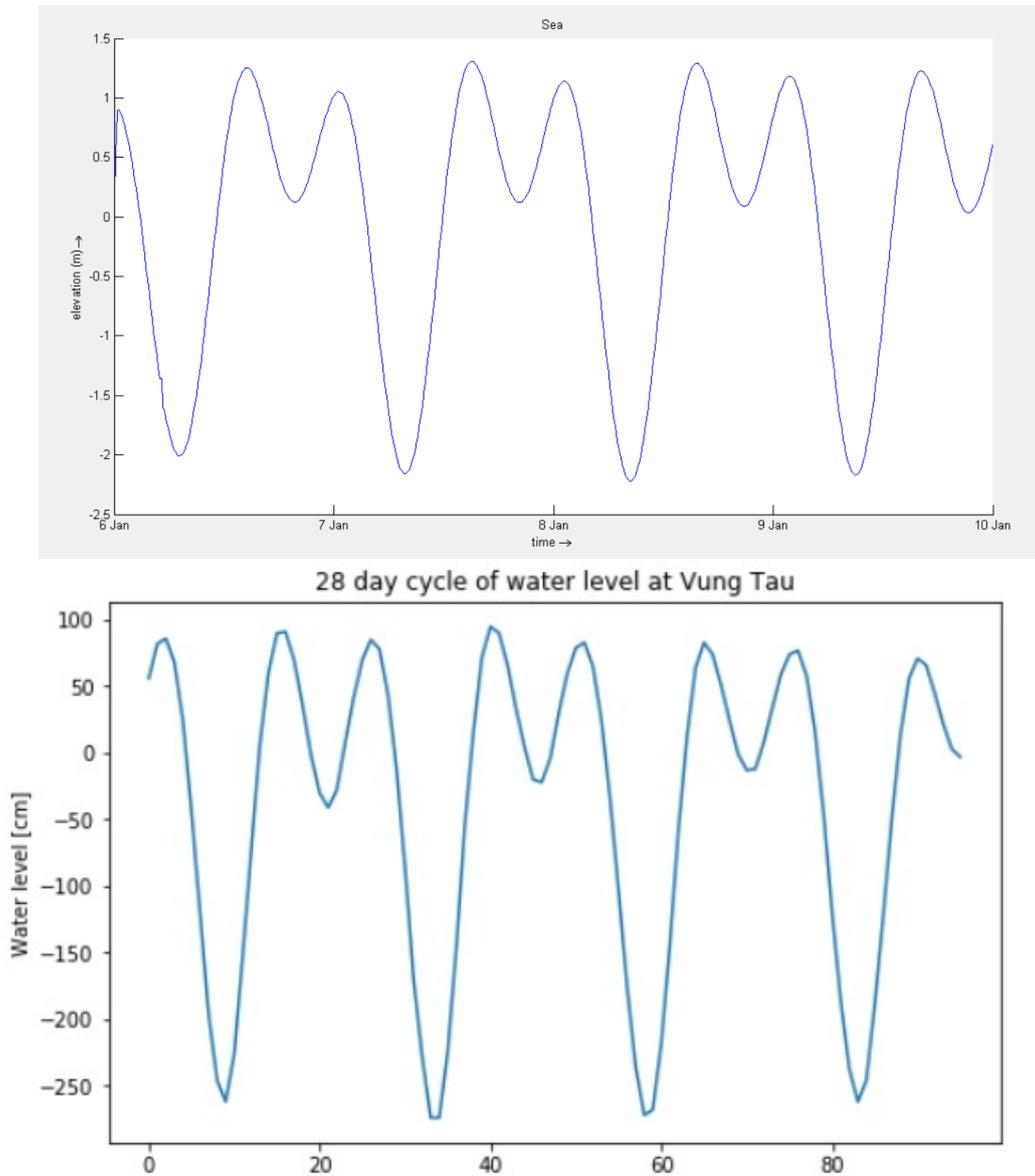
Figure 4.10: Validation tidal output Delft3D with measured data
