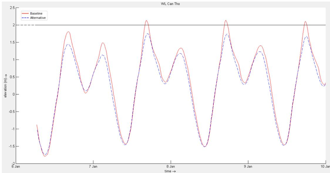
Figure 6.24: The calculated water level in Can Tho baseline and with the bypass channel
