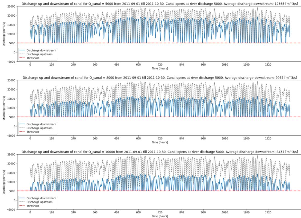
Figure 6.22: Results of using a bypass channel with different discharges
