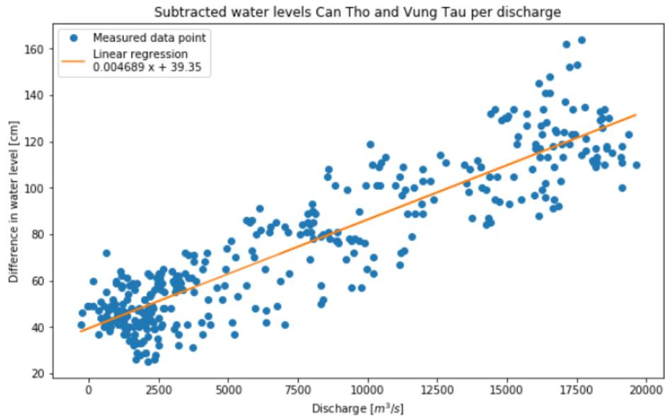
Figure 4.3: Linear regression for discharge and differences
