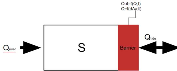
Figure 4.6: Zero-dimensional model discharge sluice schematic
