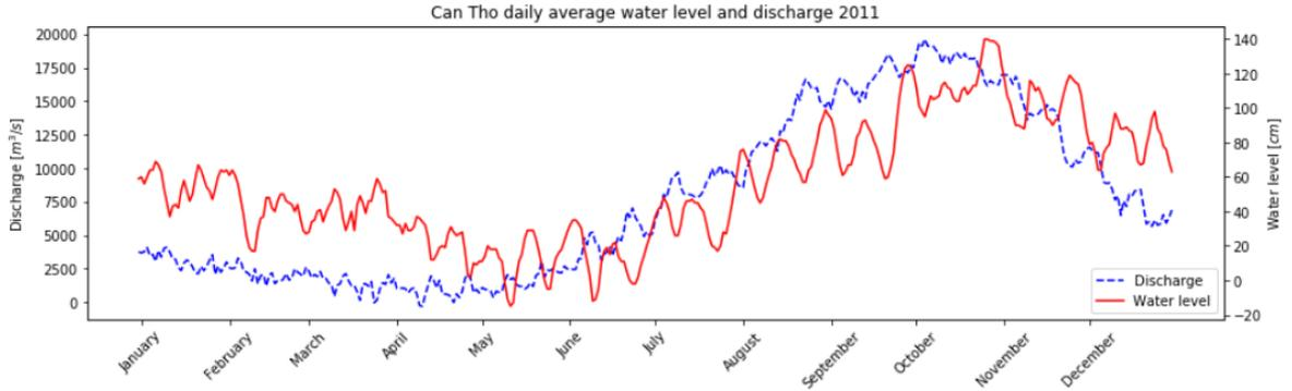
Figure 3.10: Daily discharge and water level at Can Tho (“SIWRR dataset”, 2011)
