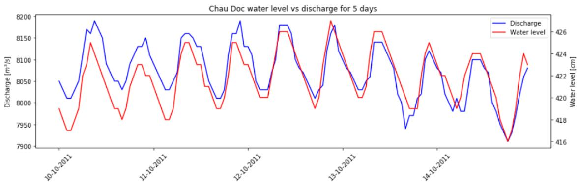
Figure 3.9: Hourly discharge and water level at Chau Doc in October
