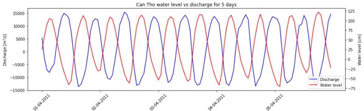
Figure 3.7: Hourly discharge and water level at Can Tho in the dry season
