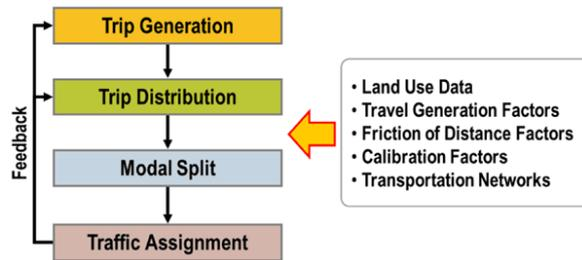
Figure 4.12: Four-step model (Rosenbaum & Koenig, 1997)
