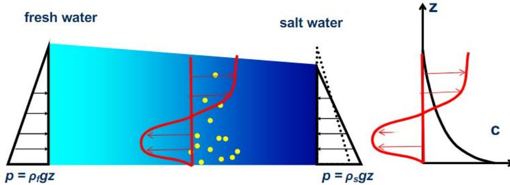
Figure 6.2: Salt water intrusion during ebb (van Prooien, 2022)
