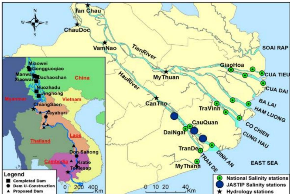
Figure 3.1: Measuring stations in the MKD (MAI et al., 2018)
