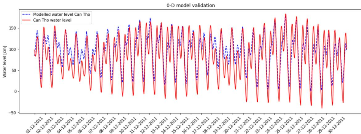
Figure 4.4: Calculated water levels in Can Tho for December
