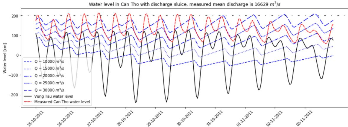
Figure 6.4: Change in water level for different discharges,  $S = 200 \text{ km}^2$
