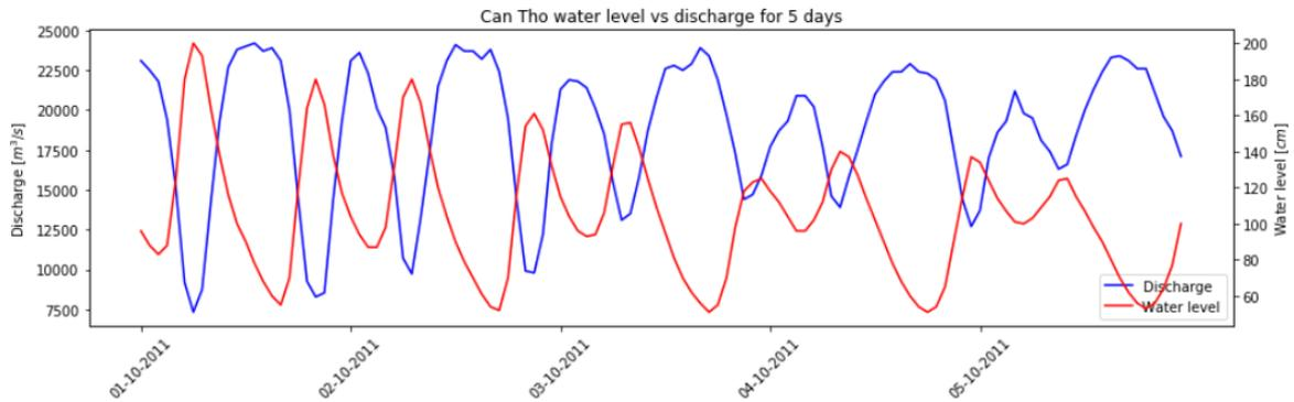
Figure 3.8: Hourly discharge and water level at Can Tho in October
