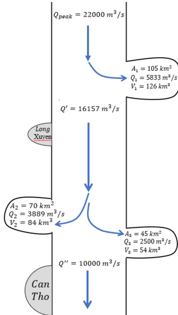
Figure J.1: Schematisation of the Hau River after reestablishing wetlands
