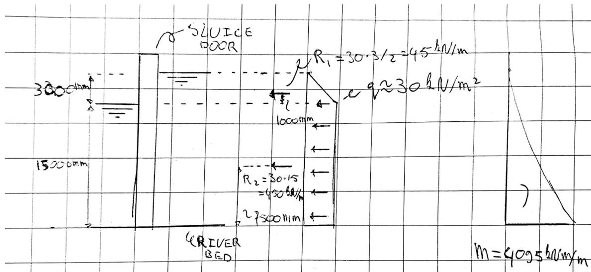
Figure I.2: Schematisation of the discharge sluice side view
