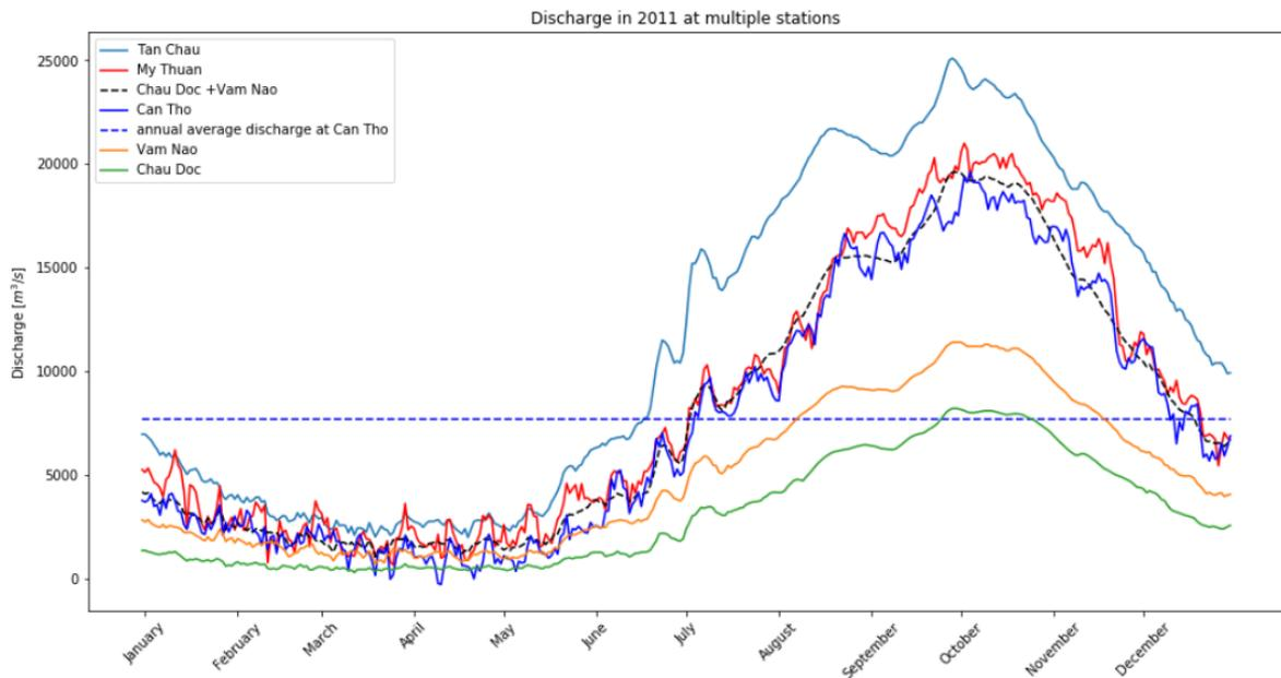
Figure 3.3: Discharge at all measuring stations
