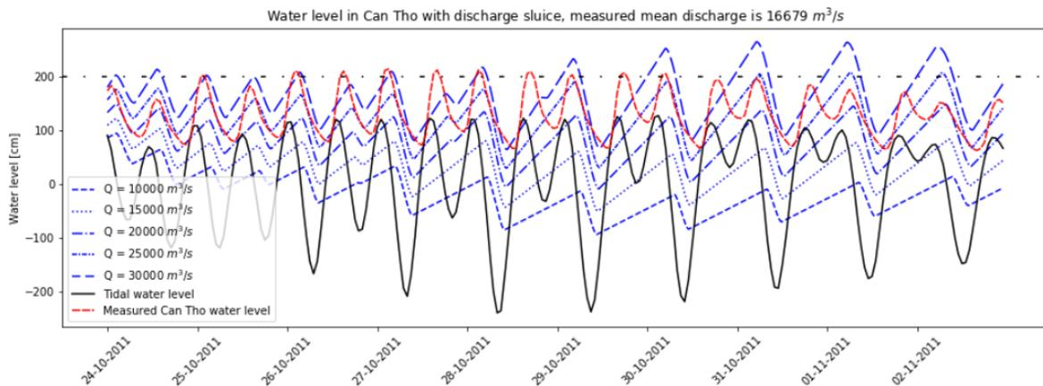
Figure 6.3: Change in water level for different discharges,  $S = 80 \text{ km}^2$
