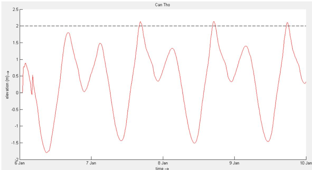
Figure 4.9: The water level at Can Tho relative to the flood threshold of 2.0 meters
