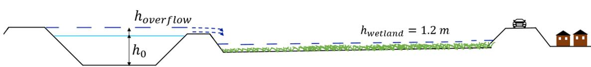
Figure 6.14: Schematic cross-section design of the double levee system
