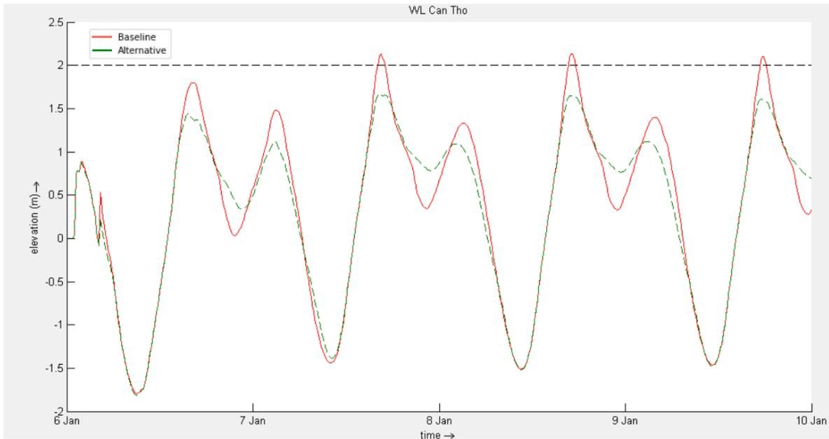
Figure 6.16: The calculated water level in Can Tho baseline and with wetlands
