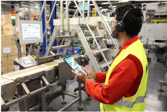
FIGURE 1. An operator interacting with the cognitive assistant by voice and graphical user interface.
