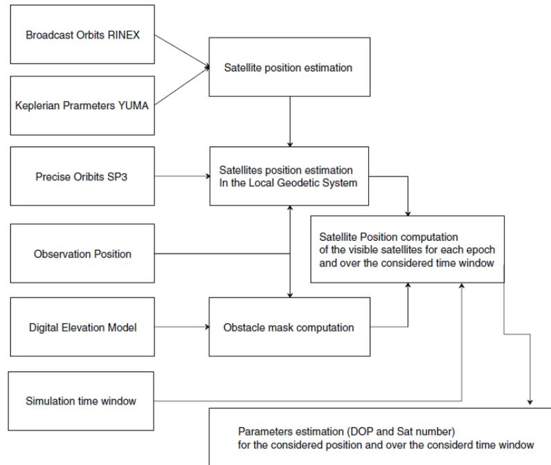
Figure 5: Flowchart of the software (Gandolfi et al. 2011)
