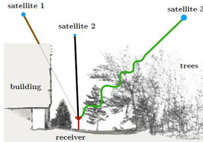
Figure 2: Complex environment in the case of satellite visibility ([Dandurand et al. 2019](#))
