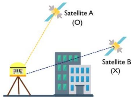
Figure 1: Signal obstruction from satellite to receiver ([Lu et al. 2020](#))
