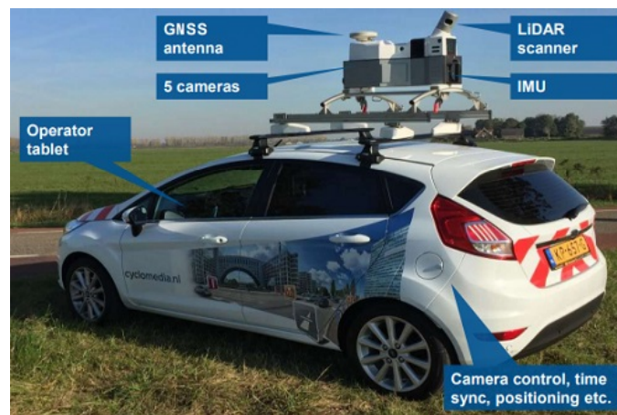
Figure 3.1.: HD-Cyclorama recording system: DCR10.
