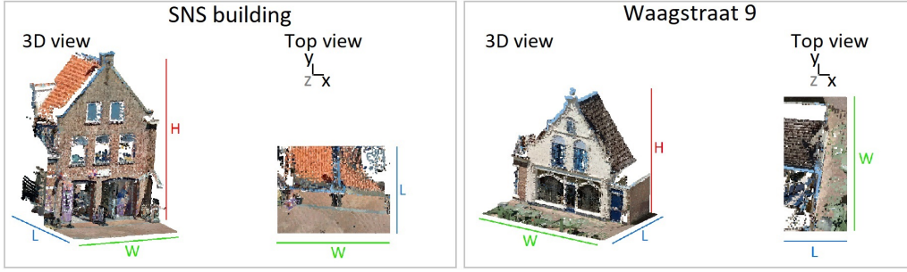
Figure 2.13: Left, a building with the width in x direction and right a building with the width of the building in y direction.
