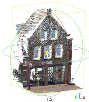
Figure 2.15: Bounding box of the data of a single building. The center of the points is displayed with a yellow dot.
