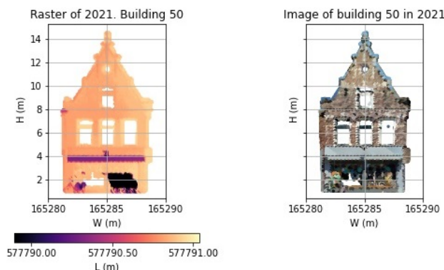
Figure 5.4.: From left to right, raster containing the length component of the data points of Voorstraat 50, and an image of the building.
