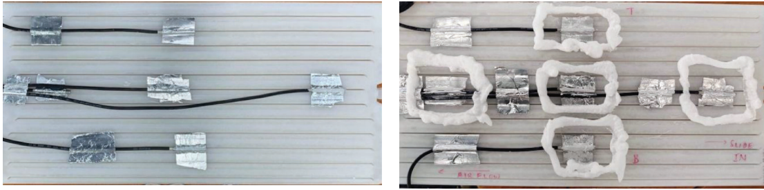
(a) Sensors are held in place with a metallic conducting tape to measure the surface temperature of the adjacent PCM panels.
