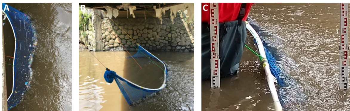
Figure 5.2: Water level difference between up and downstream of the big net filled with 5 minutes of accumulated debris at measurement location 2 on 16/05/2018.
