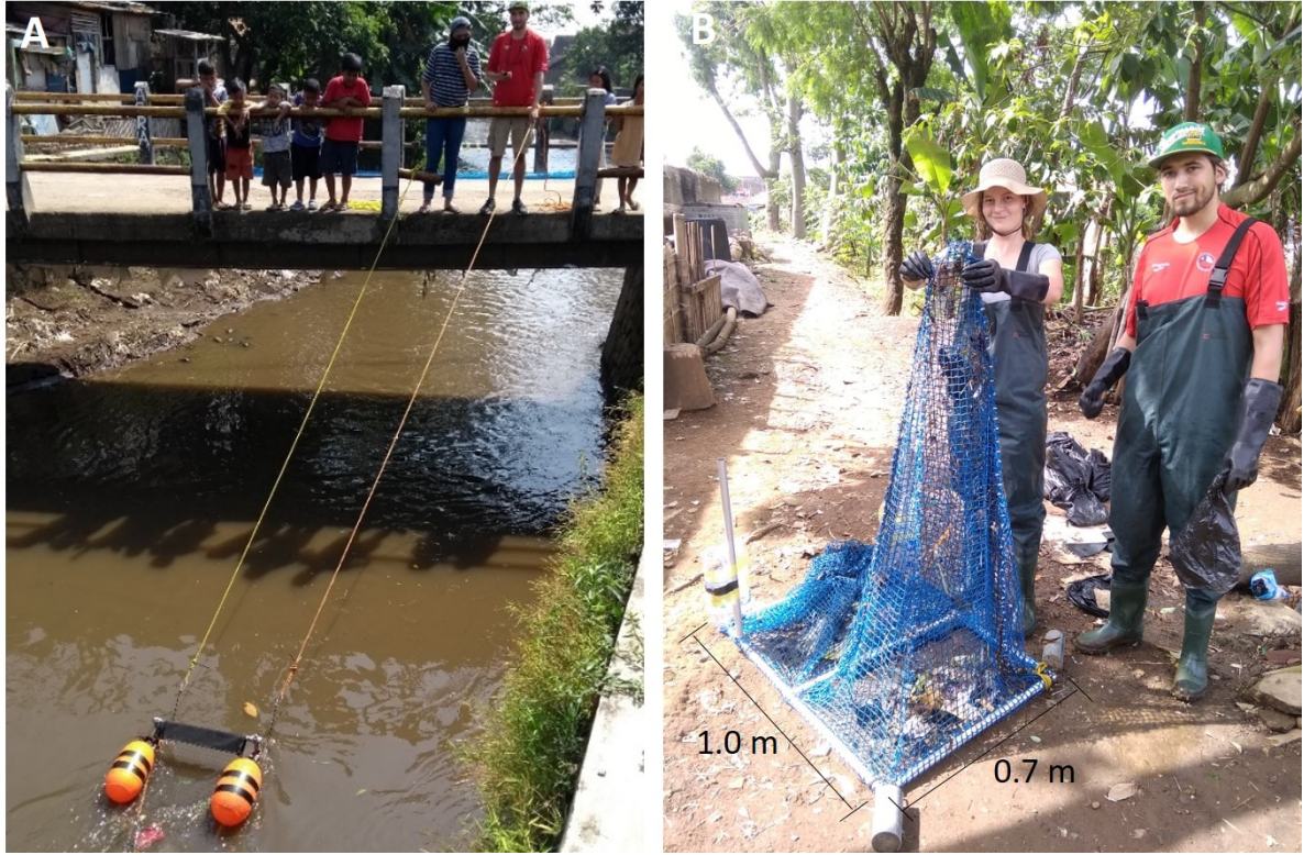
Figure 5.3: (A) Trawl measurement set-up at measurement location 2 and (B) emptying the double trawl measurement before sorting.
