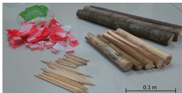
Figure 6.1: Examples of the five different types of debris; large vegetation, medium vegetation, small vegetation, straws and plastic bags.
