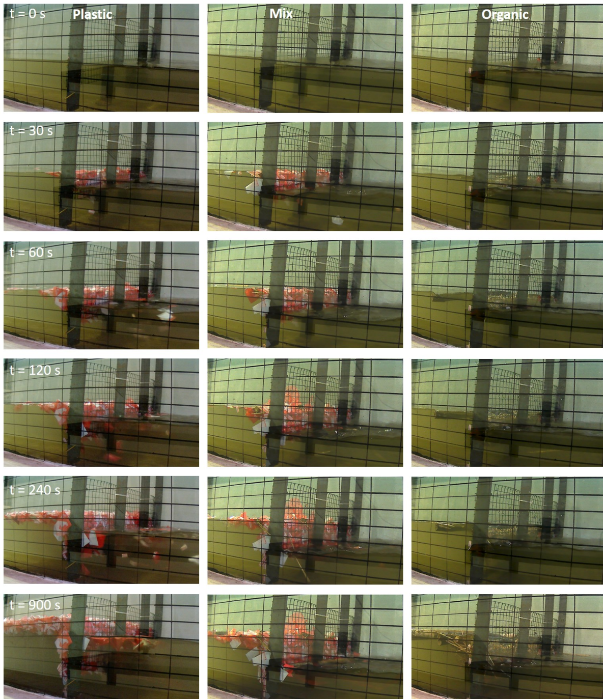
Figure 6.3: Comparison of the debris accumulation growth over time at trash rack for plastic debris (test 4), a mixture of organic and plastic debris (test 7) and organic debris (test 1), with a debris weight of 0.8 kg and an approach flow velocity of 0.4 m/s.
