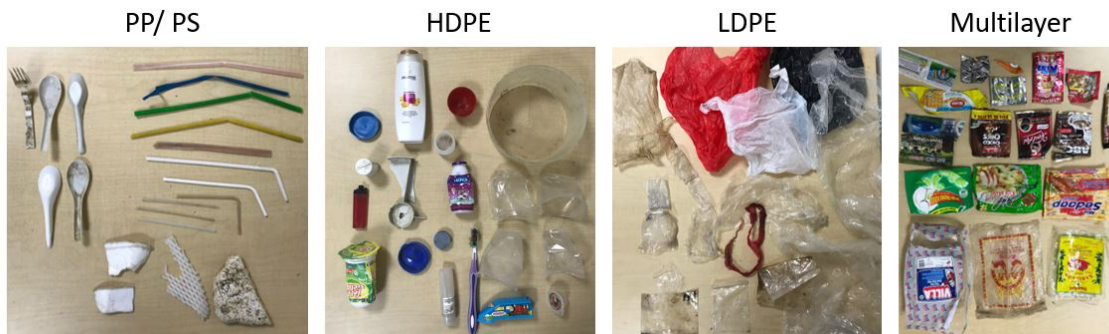
Figure 5.9: The 20 samples of the four plastic categories; PP/PS, PO Hard, PO Soft and multilayer, that were taken back into the laboratory to compare the dry and wet weight.
