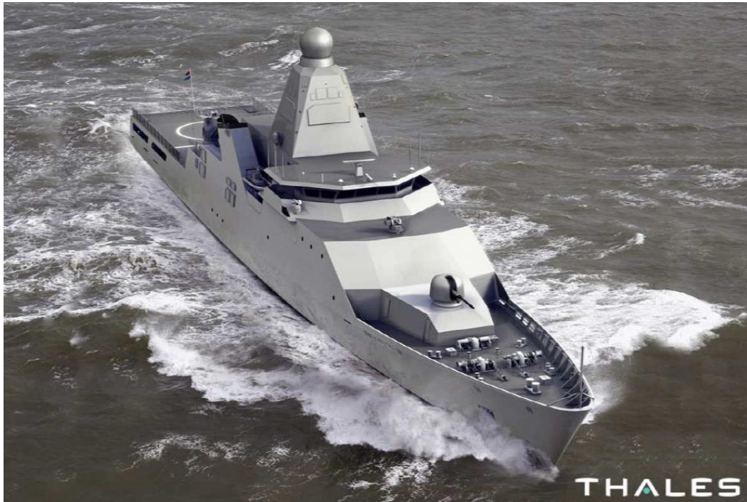
Fig. 4.1. A photo of a Thales integrated mast, seen on top of the naval vessel, containing all major radars, sensors, and antennas.
