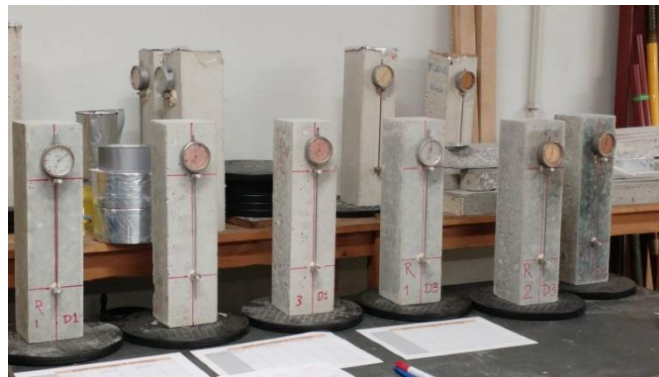
Fig.8 Drying shrinkage test setup
