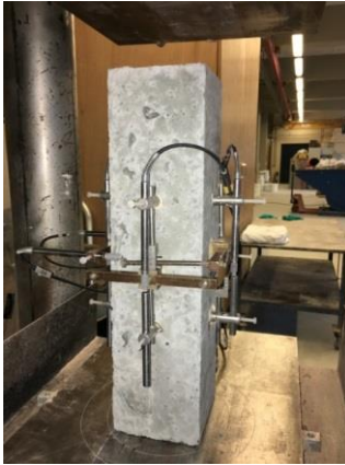
Fig.6 E-modulus test setup
