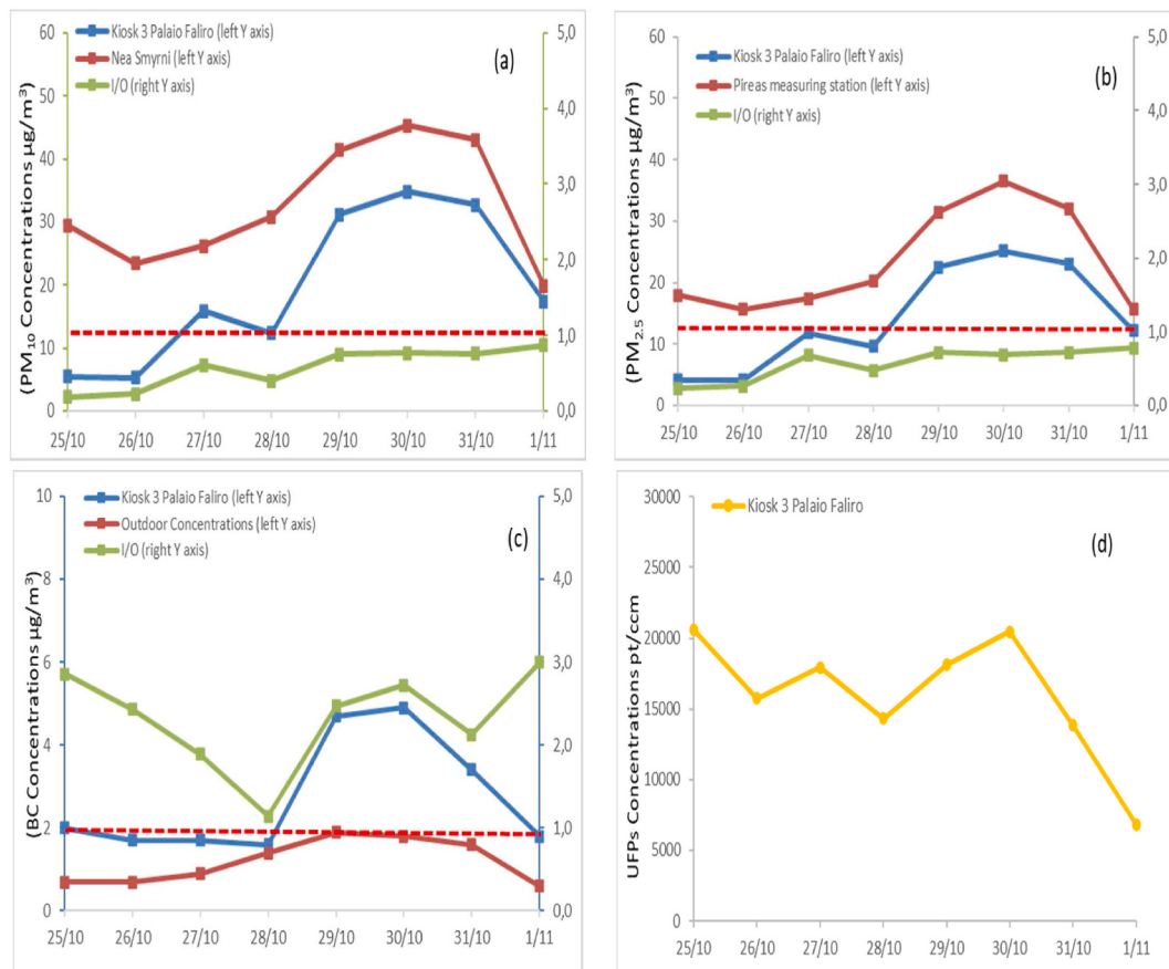
Fig. 8. Daily average concentrations recorded indoors in the Kiosk 3 (Palaio Faliro) and outdoors during the sampling period (a) \text{PM}_{10} concentrations (b) \text{PM}_{2.5} concentrations (c) BC concentrations (d) UFPs concentrations.
