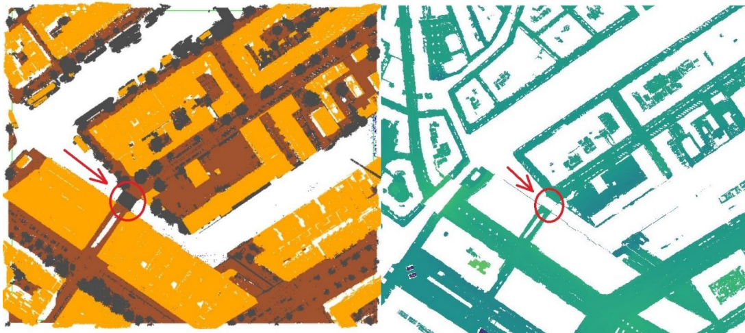
Figure 2.7: AHN3 raw point cloud (left) and DTM raster (right). Bridges are not included in the DTM raster.
