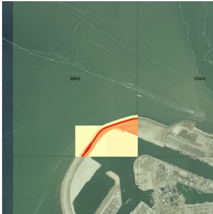
Figure 3.3: Image showing how this DTM along the coast is only partially water flattened
