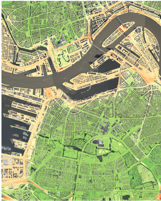
(a) "Swiss cheese" DTM with many holes and no-data values for buildings and water
