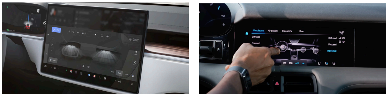
Fig. 7 - The interfaces to control the air conditioning vents in a Tesla and a Porsche Taycan (Tesla & MKBHD)
