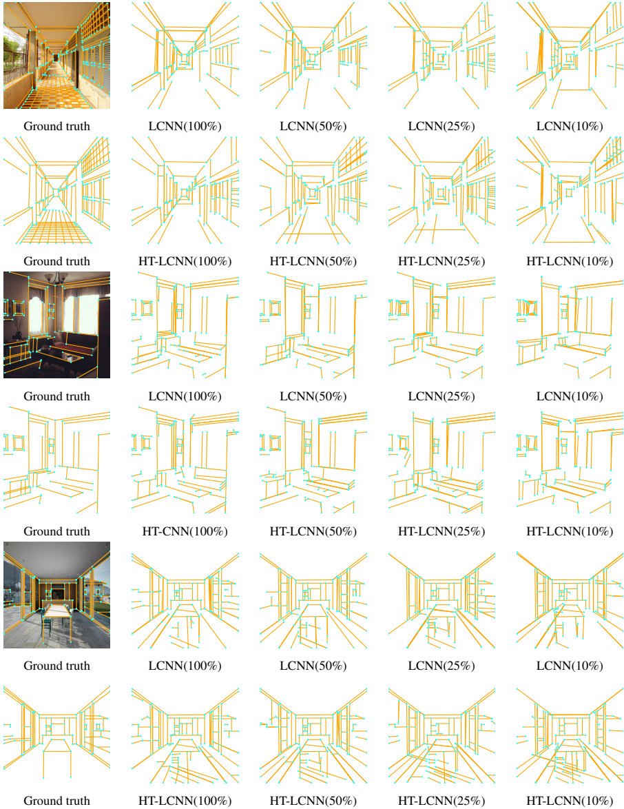
Figure 2.12: Exp 3.(a) : Visualization of detected wireframes from HT-LCNN (9.3M) and LCNN (9.7M) [6] trained on various Wireframe subsets [5]. Our HT-LCNN can more precisely detect the wireframes of the windows than LCNN, as shown in the first example. However, our HT-LCNN generates more false-positive predictions from the shadow of objects, when compared to LCNN, as shown in the last example.
