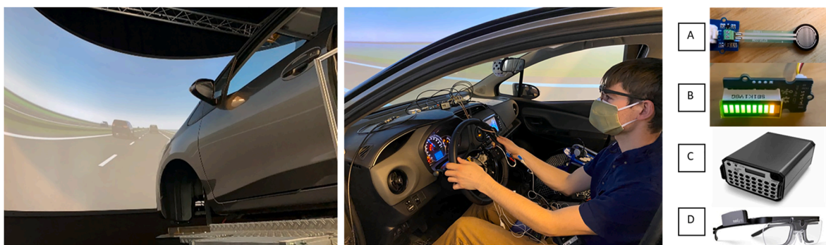
Fig. 1. Experimental setup. Left side: Driving simulator (DAVSi) at Delft University of Technology. Middle: Participant with all measurement devices. Right side: (A) Pressure sensor for reporting continuous perceived risk. (B) LED bar- visual feedback of reported continuous perceived risk. (C) ECG device TMSi to measure cardiovascular activity. (D) Eye tracker Tobii pro 2 to measure pupil dilation.
