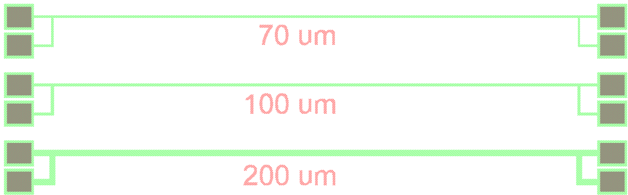
Figure 13 Test structure for bending test. The green color represents the graphene and the red color represents metal layer.
