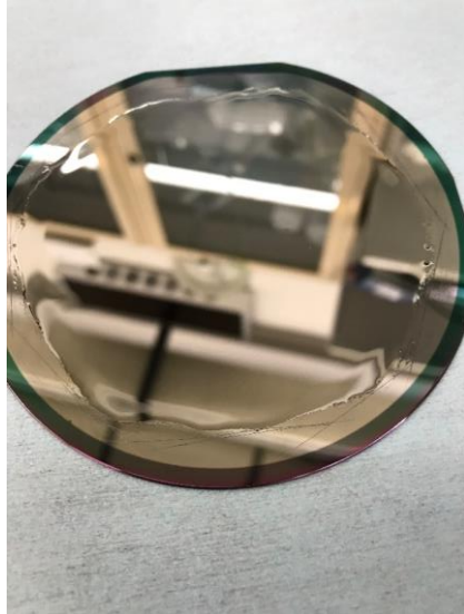
Figure 42 The test wafer for the nickel lift-off process. Incisions were made around the PDMS to break the silicon dioxide sealing.
