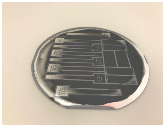
Figure 82 The test wafer after the PDMS etching process
