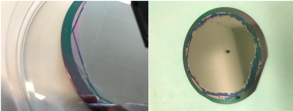
Figure 43 (left) Close-up on the incision after the wafer is submerged in water. (right) The test wafer after the peeling attempt.
