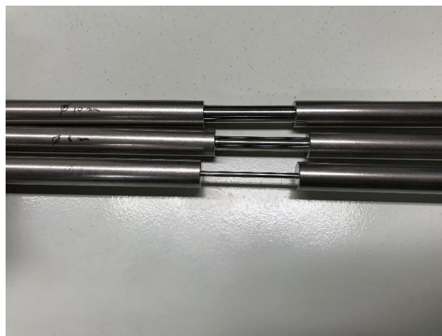
Figure 7 Metal rod for controlling the bend radius
