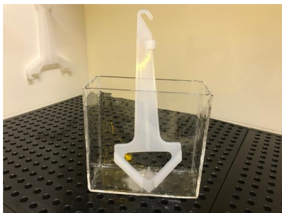
Figure 48 The glassware and wafer carrier used in the separation process.
