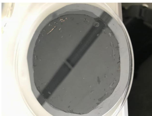
Figure 49 Target wafer after delamination process of the etch and pick process.
