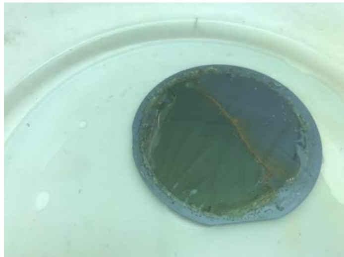
Figure 40 The PDMS on the target wafer transferred using photoresist ring technique.
