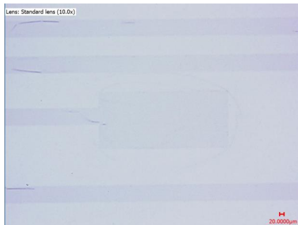
Figure 67 The remaining graphene layer after the metal mask was removed.
