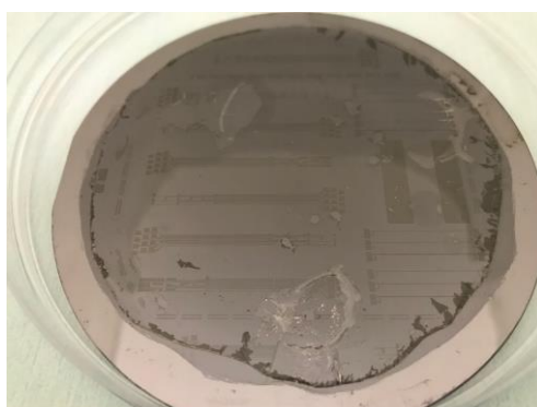
Figure 71 Overview on the graphene electrode array with no metal compensation scheme.
