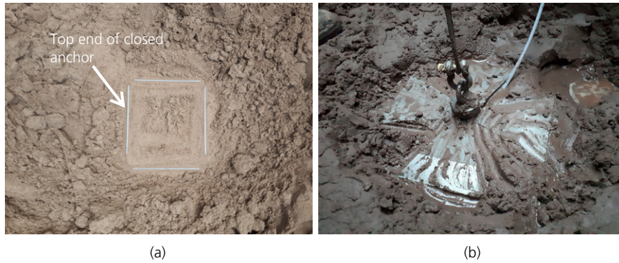
Figure 9. Photographs of the unearthed anchor: (a) closed after installation; (b) fully opened after pull-out
