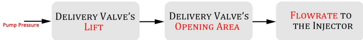
Figure 27. Conceptual Model of the 'to injector' Block
