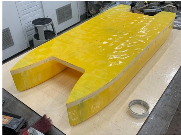
Figure C.3: Model after the final layer of epoxy
