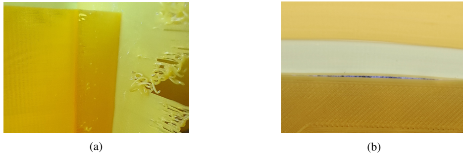
Figure 5. Common issues in areas of single-perimeter thickness: (a) Missing material near stiffeners (left); poor printing of overhanging walls (right) (b) Separation of side wall from bulkhead due to plate buckling.
