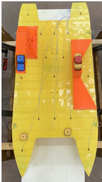
Figure 6.2: Accelerometer placements for modal experiment in air.
