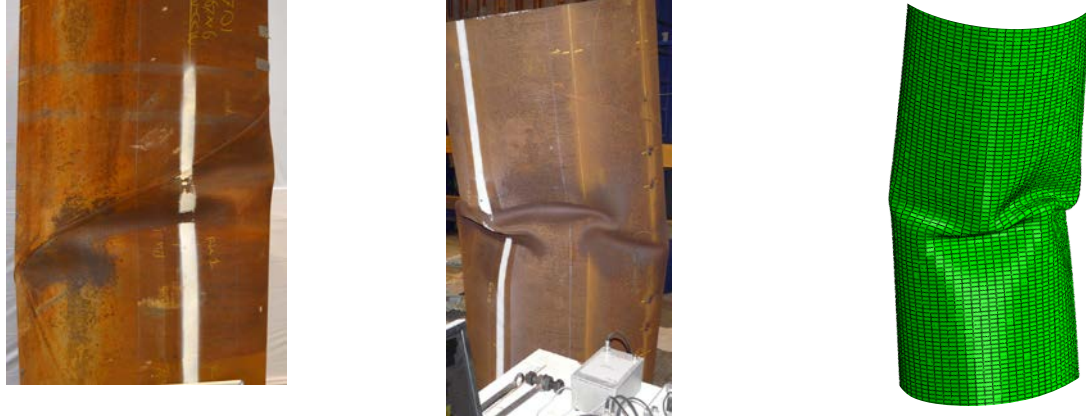
a) Test result of test T7 b) Test result of test T2 c) FEA result of test T2
