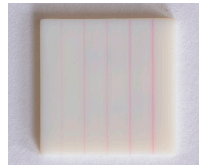
Figure 53. Sample with variation in line deepness (1 to 5 pixels deep, left to right)
