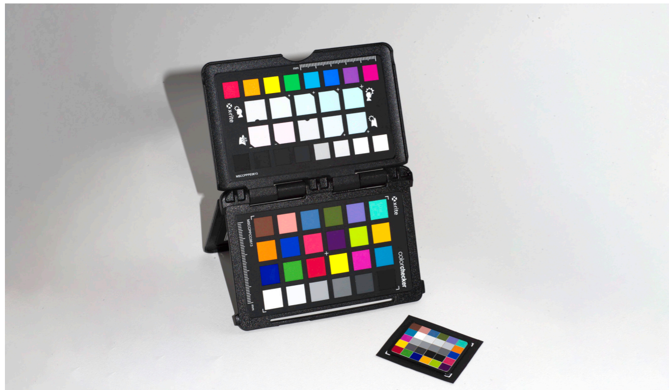
Figure 31. ColorChecker Passport and ISa ColorGauge Micro Target
