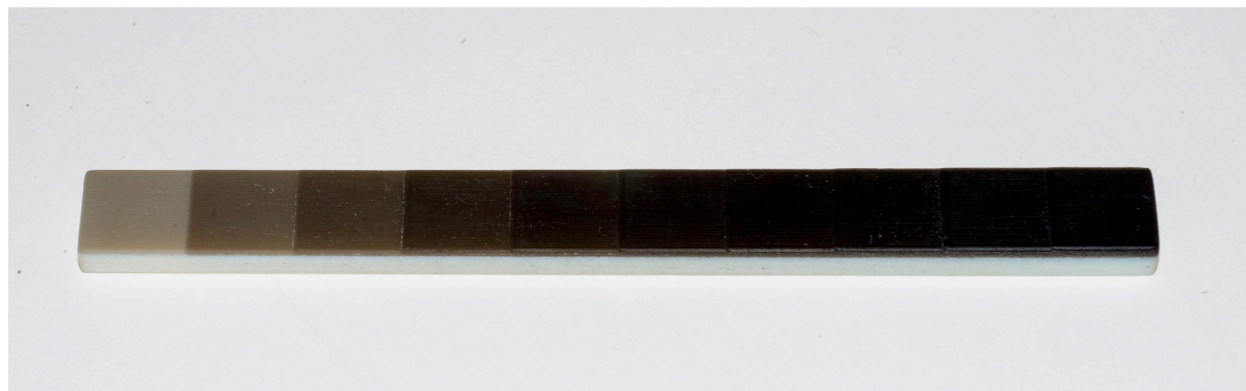
Figure 57. Black layer thickness sample, ten steps of 10 layers VeroBlackPlus (10 to 100 layers, left to right)
