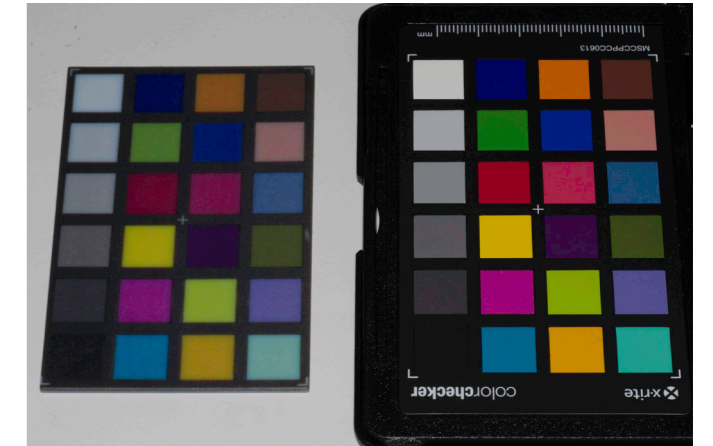
Figure 68. 3D printed ColorChecker Passport vs the original
