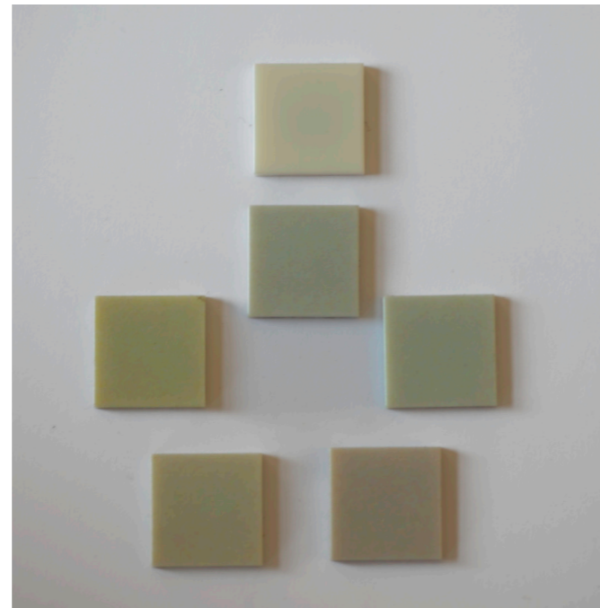
Figure 42. 3D printed sclera colour samples
