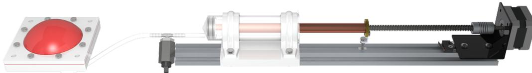
**Figure 5-4:** A single actuator module. From left to right: an inflatable membrane, a long flexible tube (longer than shown), a pressure sensor, a piston, a lead screw, a limit switch and finally the stepper motor.
