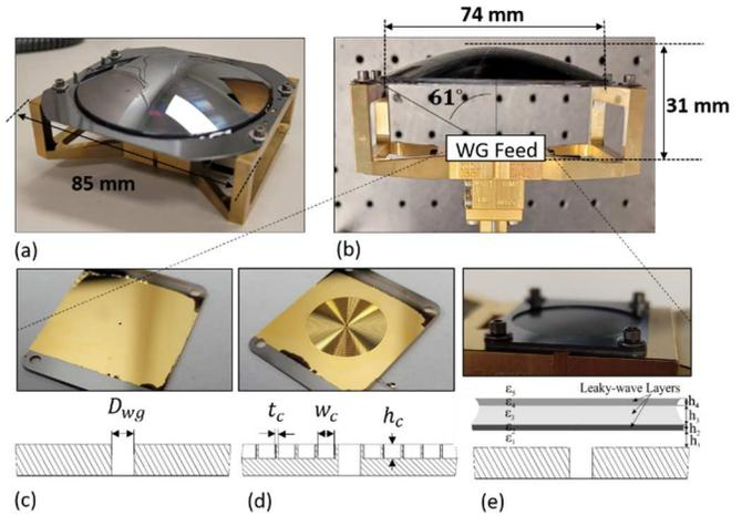
**Fig. 1.** Low profile lens antenna and WG feeds under investigation. (a) Bird's eye view of the assembled lens antenna. (b) Side-view of the assembled lens antenna; indicated is the position of the WG feed. (c) Benchmark OEWG. (d) Corrugated WG. (e) LW feed.
