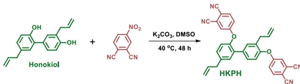
Figure 11. Synthesis of honokiol-based phthalonitrile monomer. Adapted with permission. [159] Copyright 2021, Elsevier.
