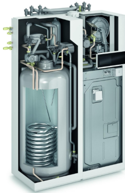
Figure 2.8: Viessmann's micro CHP unit. The tank on the left is a 220 litre hot water storage tank, the lower right part of the unit is the PEM fuel cell stack, made by Panasonic. Above the fuel cell cell stack is a gas condensing boiler for peak heat demand coverage.
