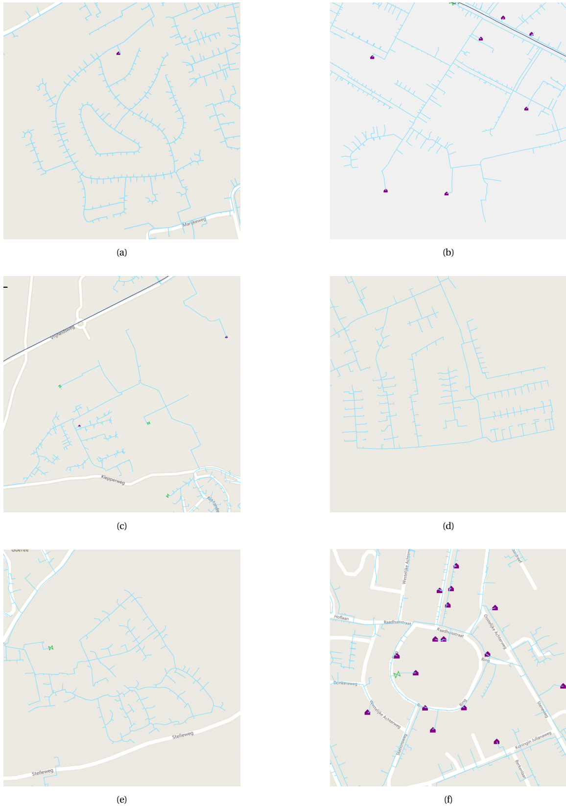
Figure 6.4: Six 100 mbar grid configurations in Goeree-Overvlakkee from software Irene PRO. The purple house-shaped icons indicate a large-scale consumer.
