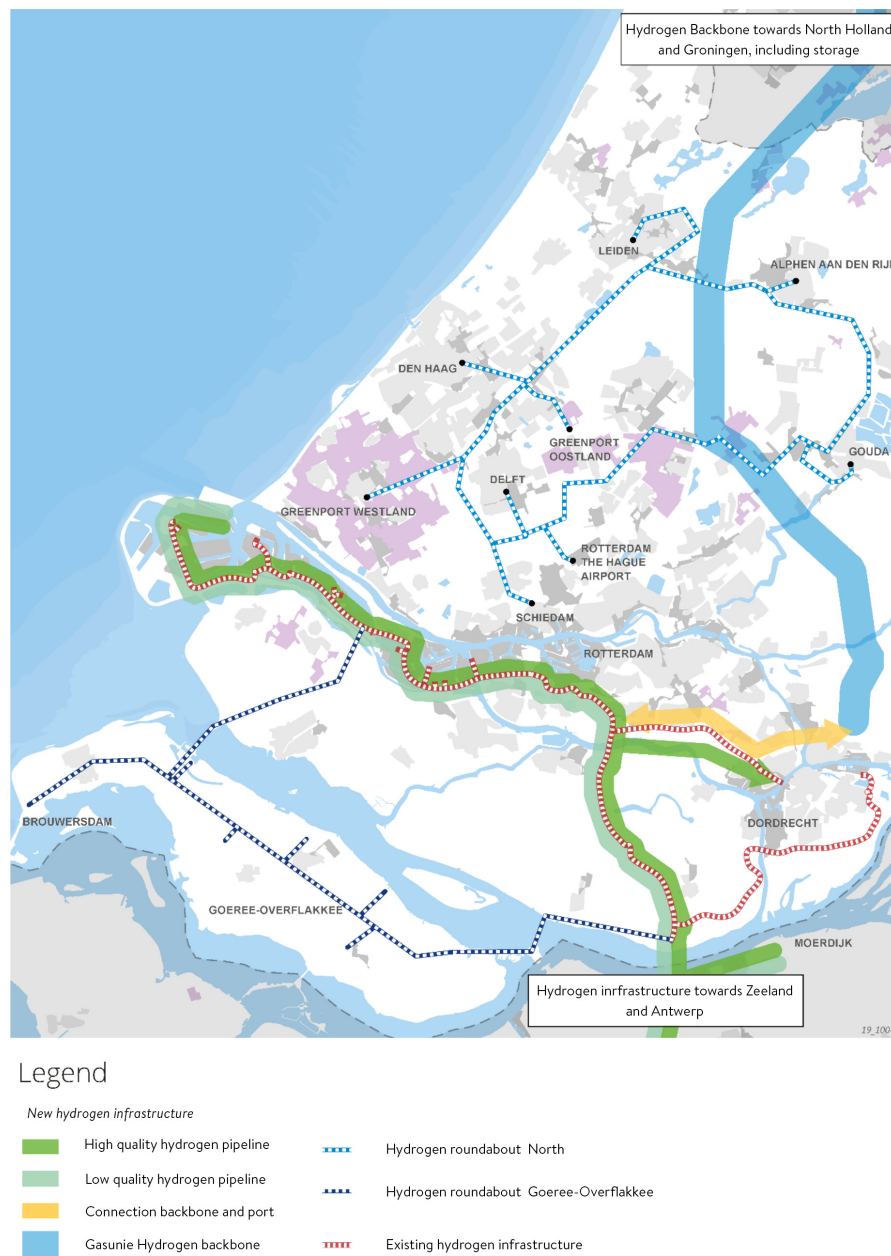
Figure 2.5: An example of a possible hydrogen infrastructure in the province South Holland, part of Stedin area. The original image was edited for translation [4].
