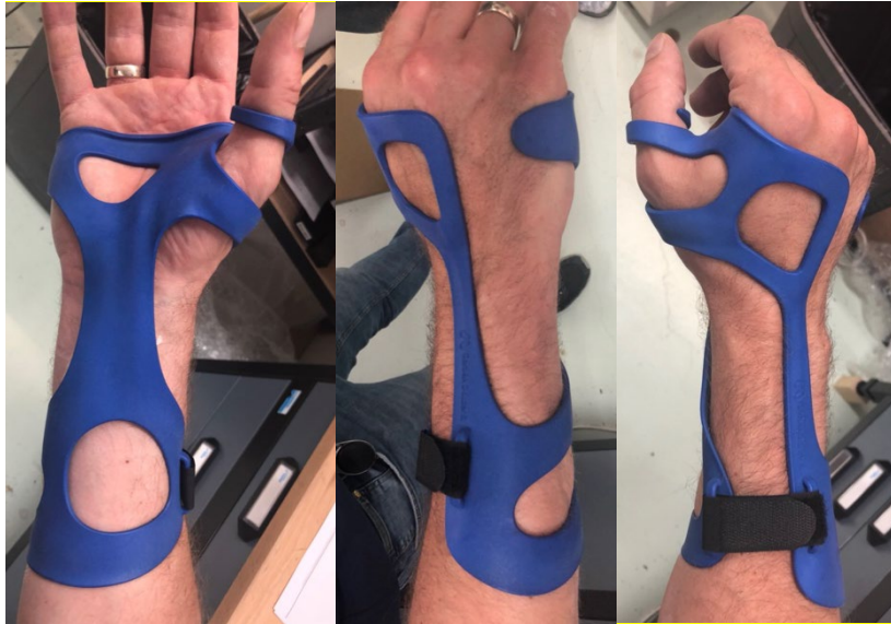
Figure 22 Fitting of the final prototype on the orthopedic technician's hand and wrist
