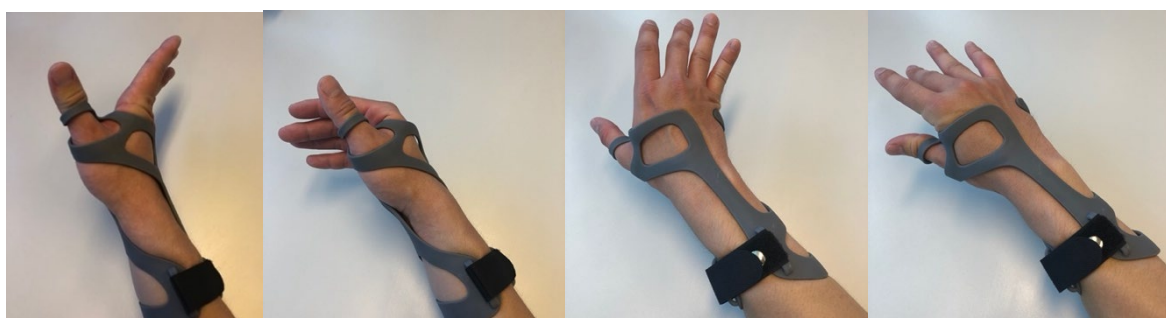
Figure 18 Behavior of the second iteration prototype while wrist motions; from the left, dorsal flexion, palmar flexion, ulnar deviation, and radial deviation. The orthosis supported all wrist motions well.
