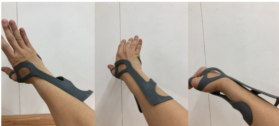
Figure 15 Behavior of the first iteration prototype while wrist motions; from the left, dorsal flexion, ulnar deviation, and palmar flexion. There were quite significant deviations that occurred while flexions were made.
