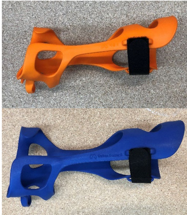
Figure 20 Final prototypes for in-house test printed in SLS-PA12. One was fitted for me (up), and the other was customized for the in-house orthopedic expert in Manometric (down).
