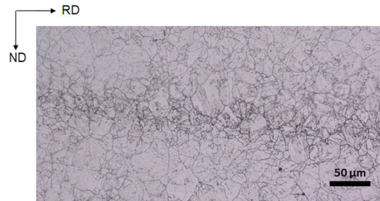
Figure 10 Prior austenite grain (PAG) distribution in the middle of the plate with the segregation band showing a reduction in PAG size in the region of the band configuring a bimodal distribution of PAG.
