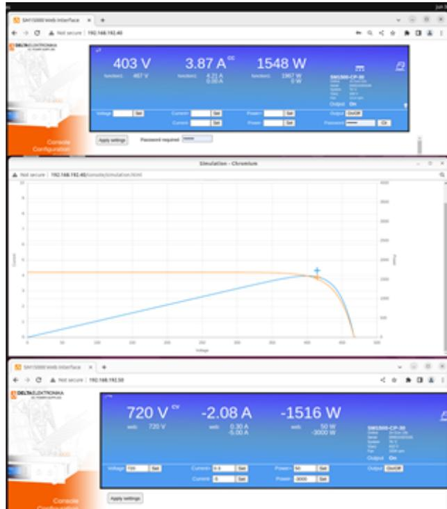
Figure 4.11: MPP Point tracking on the I-V and P-V Curves for hardware
