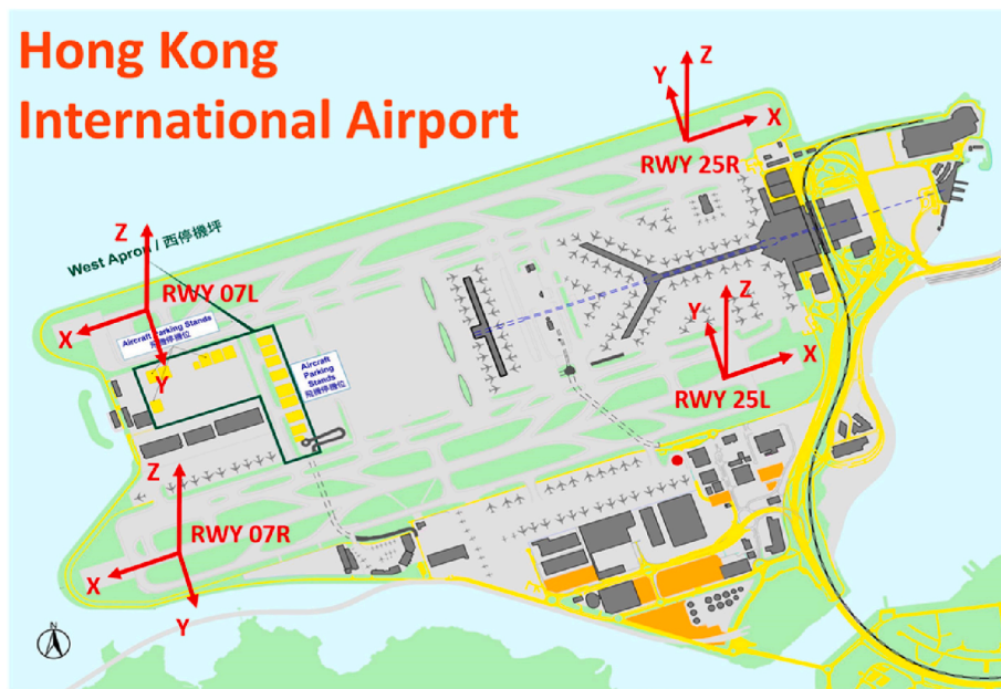
Fig. 11. Coordinate system transformation for HKIA.
