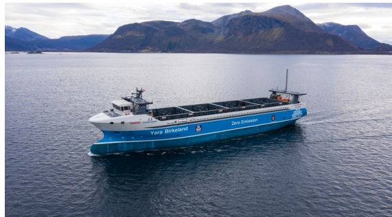
Figure 3.7: illustration of a full electric vessel, the 80 meter Yara Birkeland [Yara, 2020]
