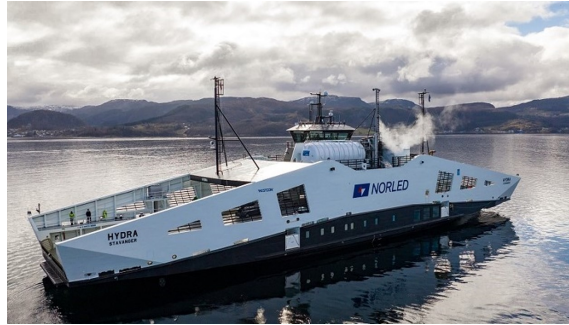
Figure 3.5: Fuel cell-battery hybrid ferry MF Hydra [NORLET, ]
