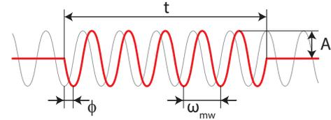
Fig. 5. Shown in red is the typical control signal required for performing a single-qubit operation; the microwave signal has a rectangular envelope of duration  $t$ . The grey line indicates the phase of the electron spin.
