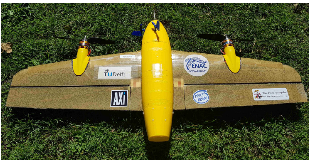
Fig. 1 The Cyclone hybrid tailsitter UAV developed at the TU Delft's MAVLab [23].
