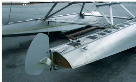
Figure 11.10: Water rudder of a float to provide control when floating on the water
