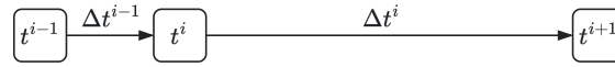
Figure 3.6: Visualisation of the meaning of the time step indices for the time and the time steps. The arrow length represents the magnitude of the time step. The blocks with the variable t inside indicate a discrete time.
