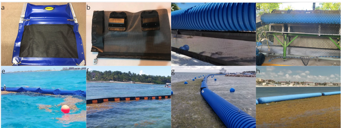
Figure 4.1: (a) Picture of type I barrier [4], (b) Picture of type II barrier [63], (c) picture of type III barrier [23], picture of type III barrier (d), (e) picture of submerged type I barrier[4], (f) picture of submerged type II barrier[58], (g) picture of submerged type III barrier[23], (h) picture of submerged type IV barrier[37].
