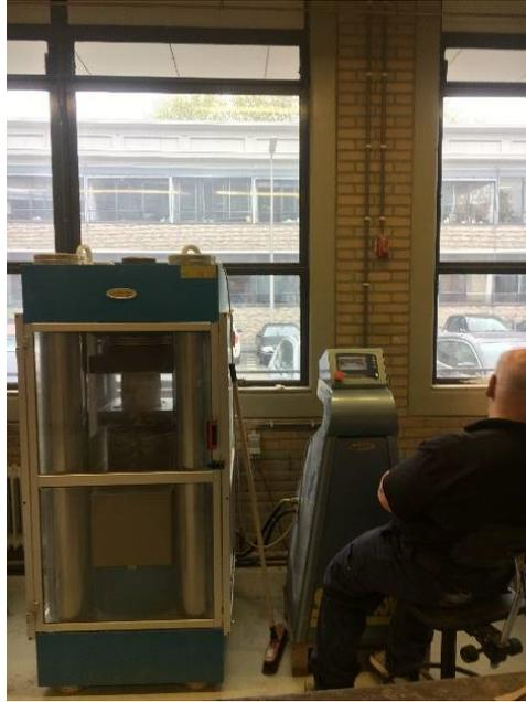
Figure 3.16: Testing of Compressive Strength of cube
