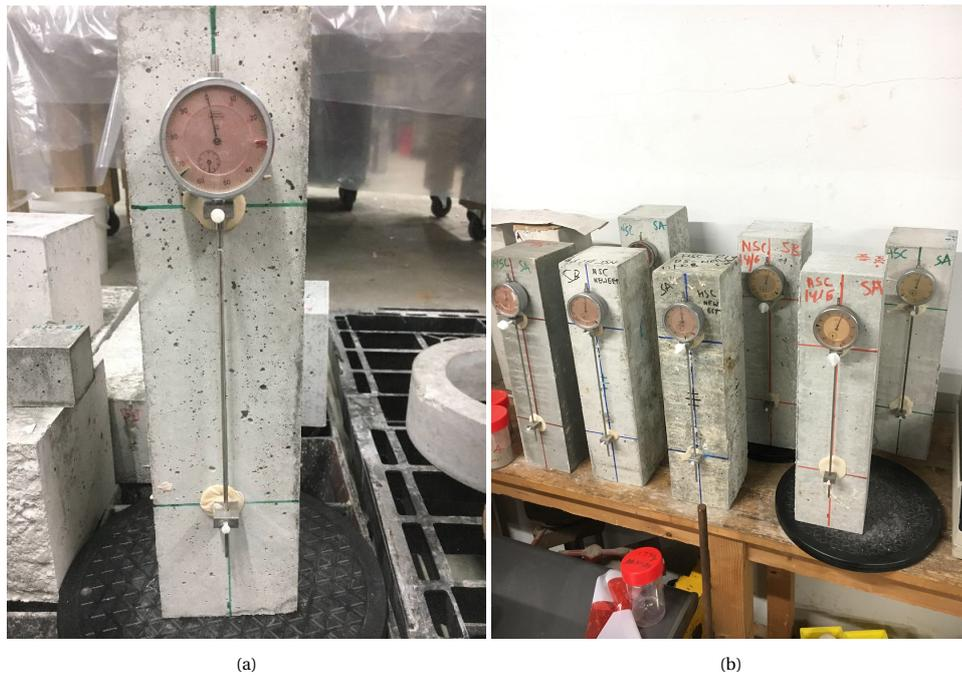
Figure 3.18: (a) Test setup for measuring Drying Shrinkage.(b) Overview of the prisms used for drying shrinkage measurement
