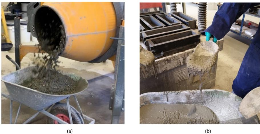
Figure 3.9: Prepared mix for (a) NSC (b) UHSC
