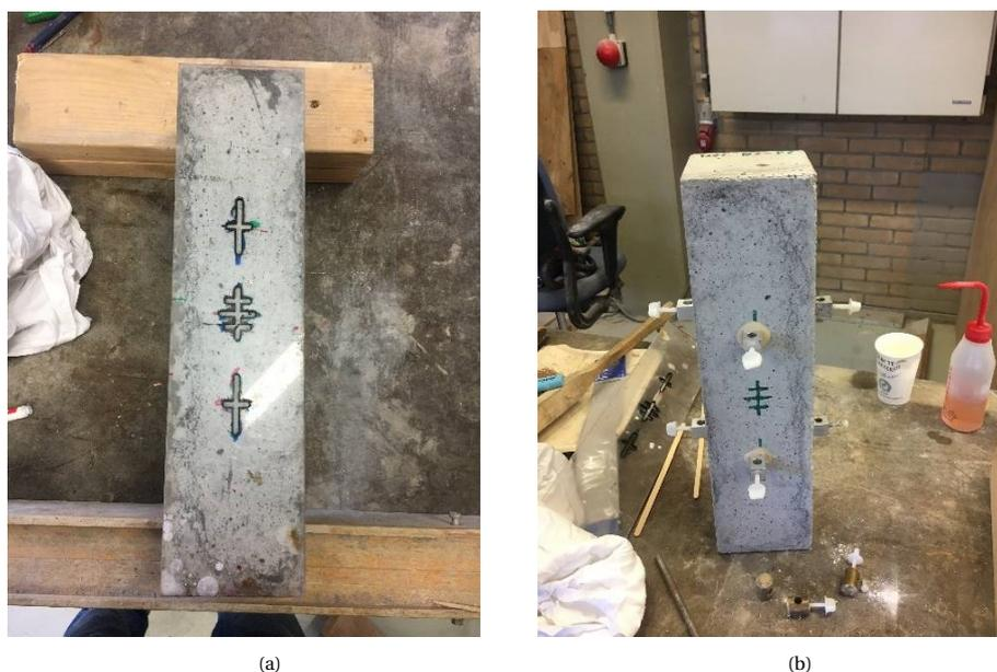
Figure 3.13: Preparation for E-modulus test (a) labelling of reference points with plastic mask (b) specimen after gluing of metallic devices
