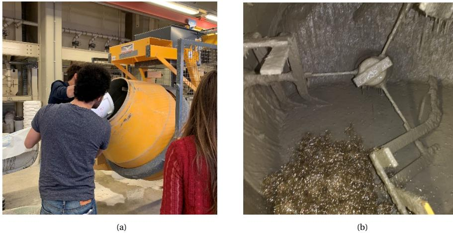
Figure 3.8: (a) Adding of water mixed with superplasticizer (b) Adding of fibres in case of UHSC mix
