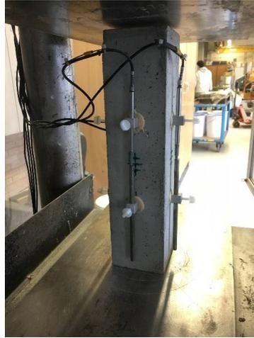
Figure 3.14: Specimen with LVDTs attached placed in the Toni Bank machine
