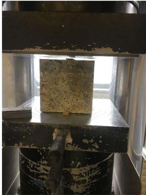
Figure 3.17: Testing of Splitting tensile strength of cube specimen
