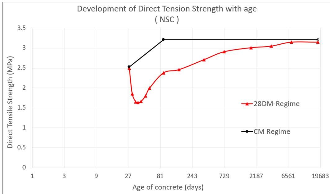
Figure 4.27: Simulation of the direct tensile strength for the NSC specimen
