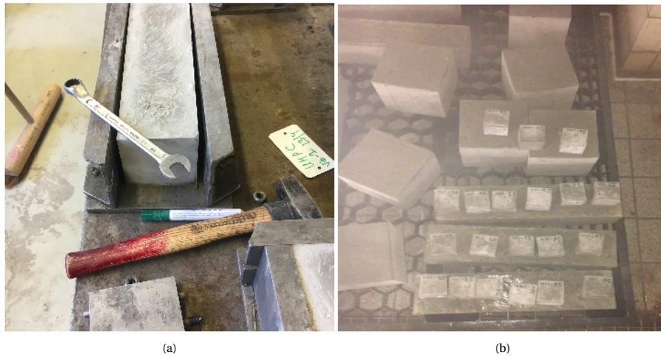
Figure 3.12: (a) Demoulding of UHSC prism (b) NSC specimens taken to the fog room
