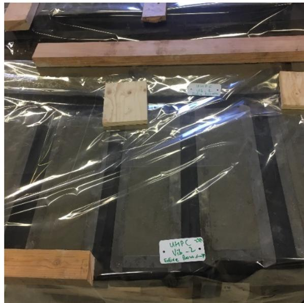
Figure 3.11: Covering of moulds with plastic sheets
